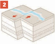
Displaced Streambed The streambed looks "broken" along its fault line.
